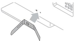
2 Pass cables through the cable management tie to avoid tangles.
